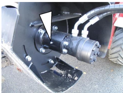
Grease nipple located on the auger and chain drive shaft
