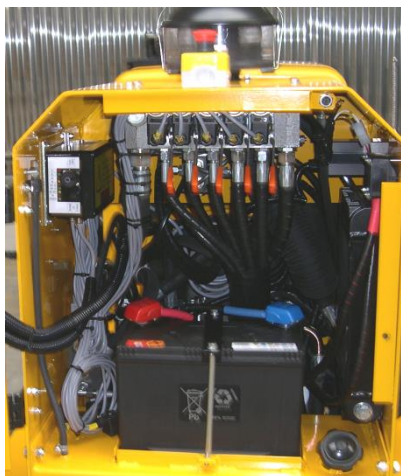
Fig. 13 - View under the rear hinged cover with battery and emergency stop button above
