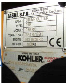
Fig. 4 – Type plates location. The machine type plate is placed together with the engine type plate.
