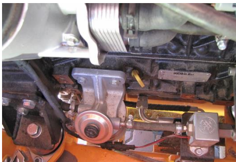
Fig. 29 – Oil level checks
