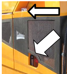
Hydraulic oil gauge with thermometer and oil filler
