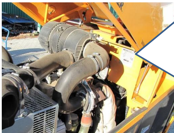
Fig. 4 – Type plates location. The machine type plate is placed together with the engine type plate.
