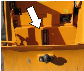
Fuel gauge – close to fuel tank filler cap
